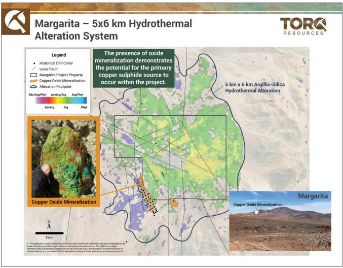
Figure 1: Illustrates the large-scale clay-silica alteration system that is centered on the Margarita property and the position of the copper oxide mineralization on the southwest corner of the project area.
